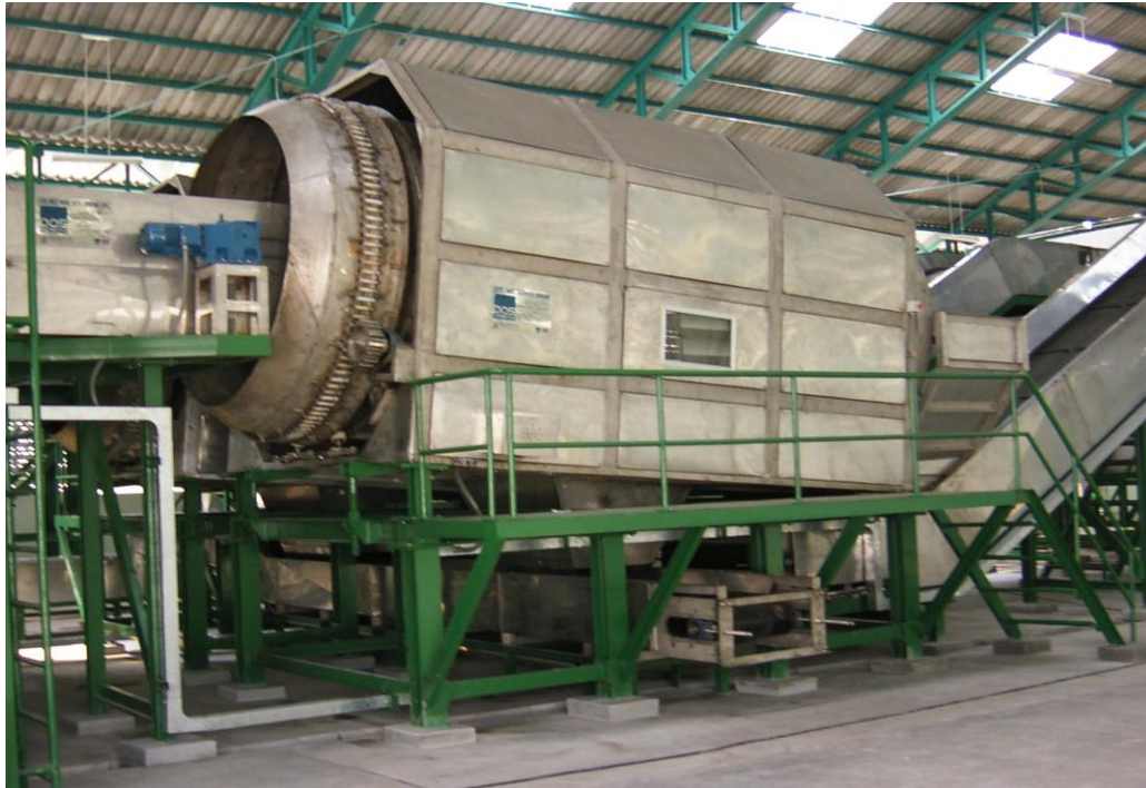
BAG RIPPER DRUM AND TROMMEL SCREEN
